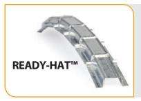
Versatile, low profile, and economical, form Ready-Hat<sup>™</sup> by hand on the job-site to the exact convex or concave shape you need. Secure it to concrete walls with power-driven fasteners or concrete nails. More than your average furring channel, Ready-Hat™ makes framing curved surfaces fast and easy.
